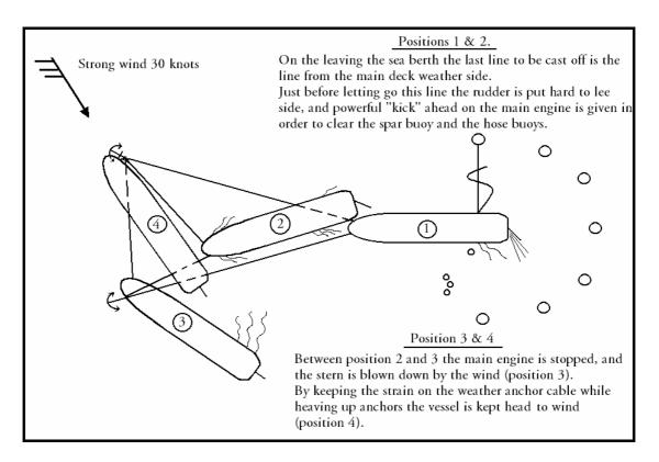
Fig. 50. Leaving the CBM with strong wind on the bow with the spar and hose buoys on the lee side.
