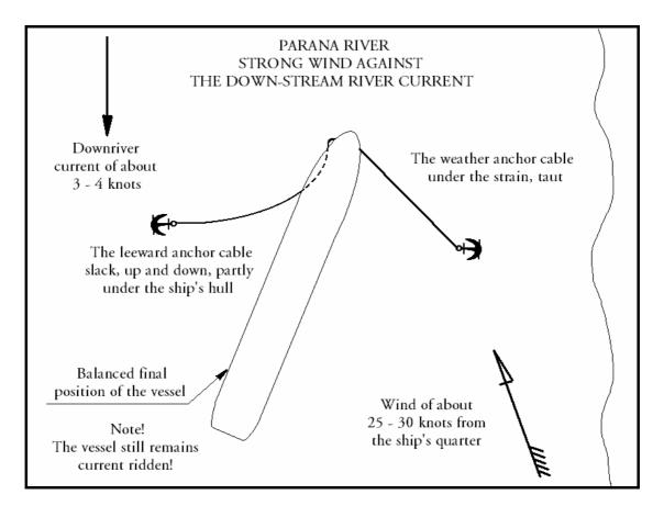
Fig. 41. Positioning of the vessel in the Parana River when strong winds are blowing from the ship's quarters.
