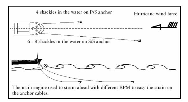
Fig. 24. Riding to two anchors.
