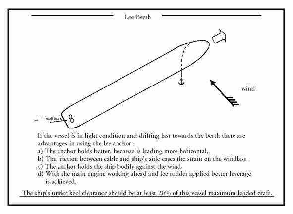
Fig. 54. Dredging lee anchor with headway.
