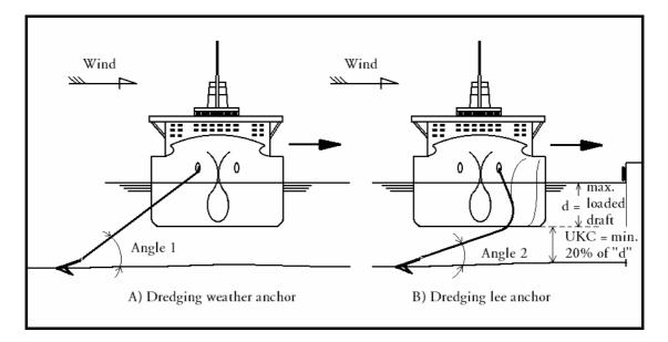
Fig. 55. Comparison of dredging weather and lee anchor.
