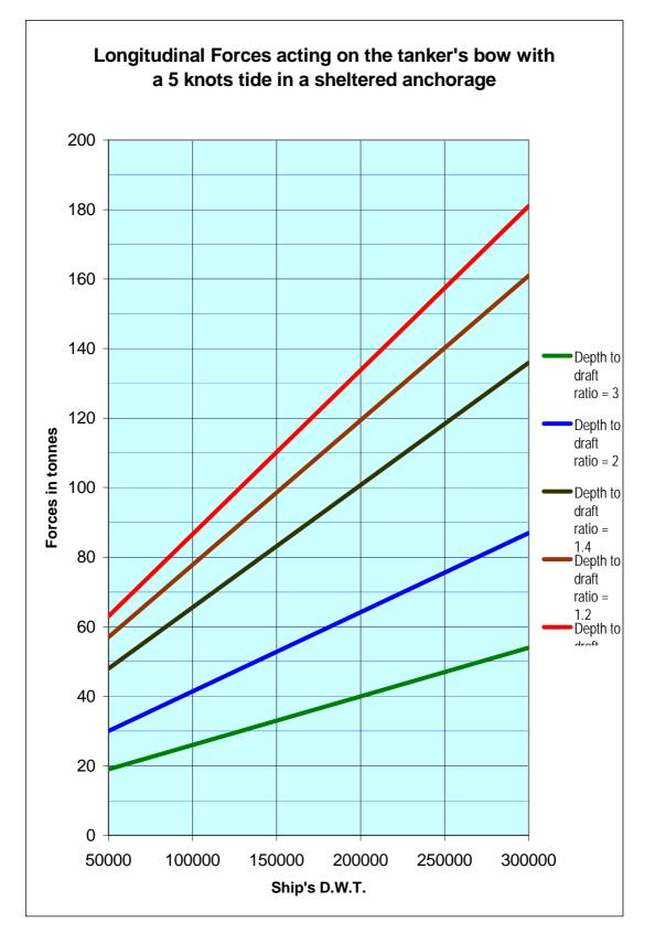
Fig. 63. Longitudinal tidal forces acting on the bow of different size vessels with a five knots tide and variable ratio of the water depth to the ship's draft.
