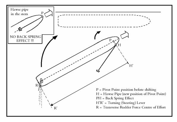
Fig. 52. Dredging weather anchor with headway. "Back Spring Effect" and Turning Lever.
