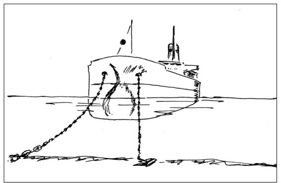
Fig. 21. The second anchor dropped "underfoot"
