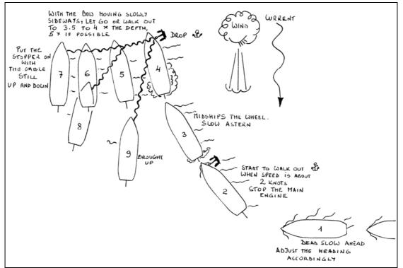
Fig. 12. The "Tentative" method (large vessels of DWT > 50,000).
