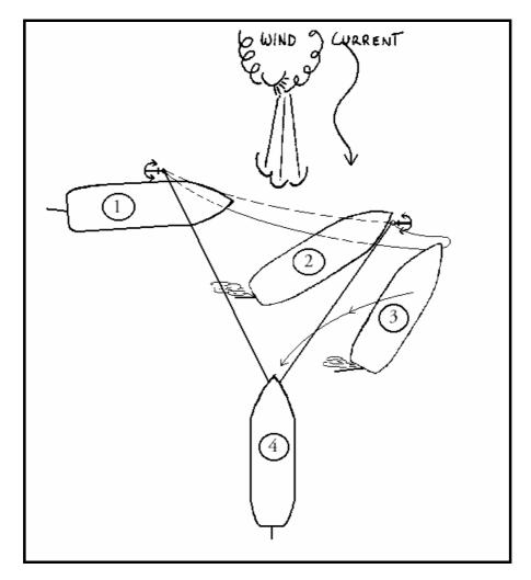
Fig. 36. The second method of carrying out "The Open Moor" manoeuvre.
