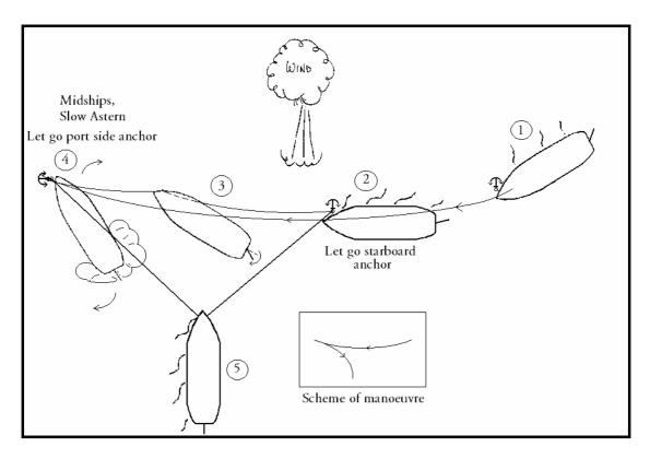
Fig. 34. Approaching to "The Open Moor" from the starboard side.
