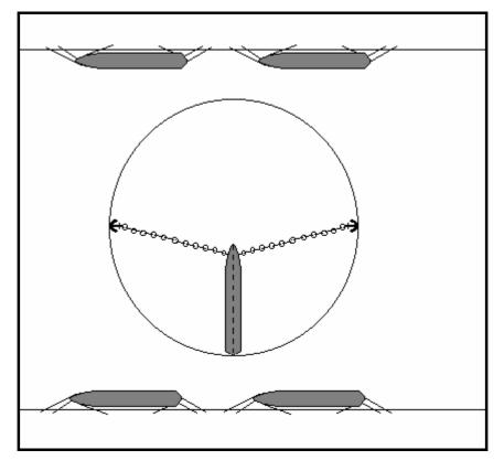
Fig. 30. Swinging room required with two anchors dropped.
