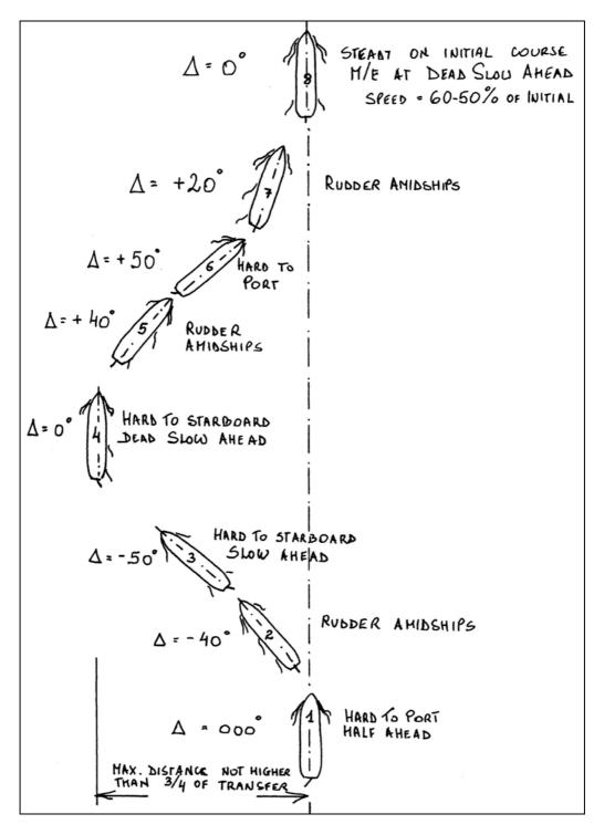
Figure 3. Rudder Cycling" or "Fish Tailing"
