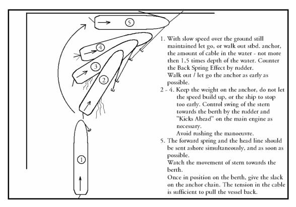
Fig. 53. Dredging weather anchor with headway.
