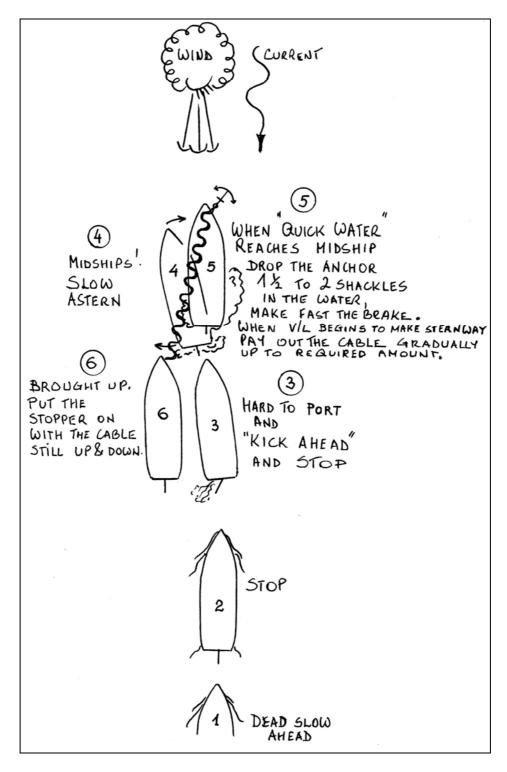
Fig. 10. The "Classic"" method - smaller vessels, up to 50,000 DWT. Water depth is up to 20 metres.
