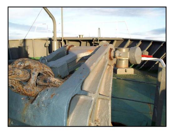
Fig. 15. Once the required amount of cable has been paid out, the vessel should be allowed to bring-up on the bow stopper. In any manoeuvring on the anchor the stopper should normally be engaged.
