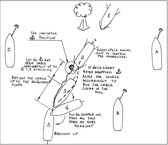
Fig. 17. Dropping the anchor with headway.
