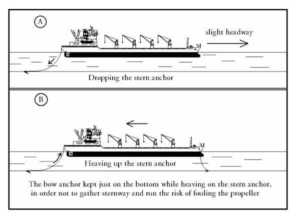
Fig. 61. The safe way of dropping and heaving up a stern anchor.
