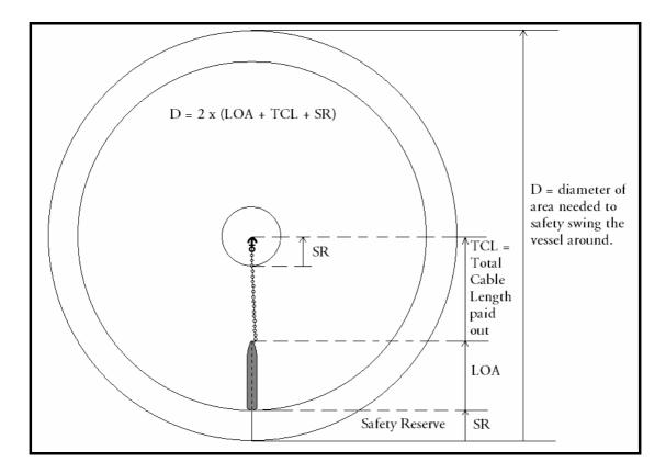
Fig. 29. Swinging room required at single anchor.
