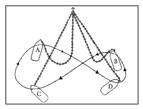
*Fig. 18. The path traced out by a starboard-anchored ship's hawse.* The anchor starts dragging or in the worst condition the cable is parted in positions where the sheer, and therefore forces are maximum.
