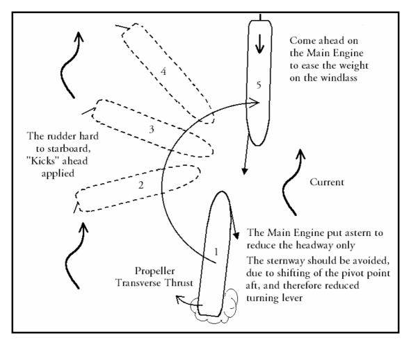
Fig. 59. Swinging to a Tide on One Anchor.
