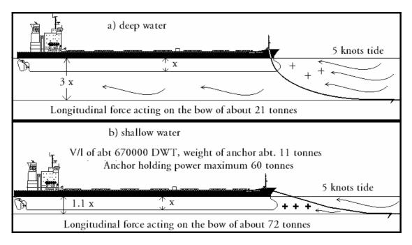
Fig. 62. Longitudinal tidal forces acting on the bow of the "Panamax" size vessel with 5 knots tide and different ratio of the water depth to the ship's draft.
