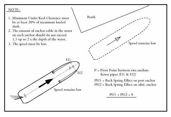
Fig. 56. Dredging two anchors with headway.
