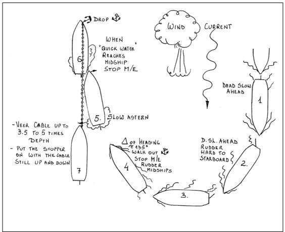
Fig. 16. The "Modified U-turn" method.
