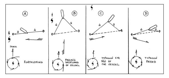
Fig. 27. "Running Moor" with 2 points on the starboard bow.
