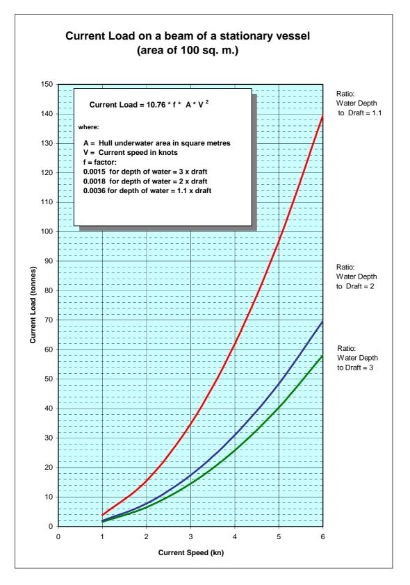
Fig. 64. Current load on a beam of stationary vessel (area o 100 sq. m).
