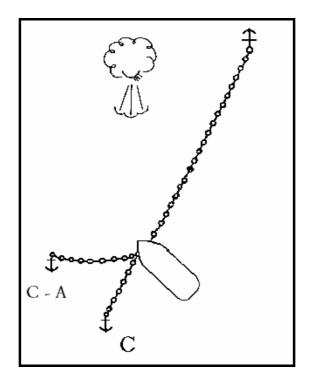
*Fig. 22. "C-A" position is better for dropping the "underfoot" anchor.* **Suggestion regarding heaving up the anchors**
